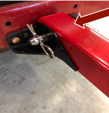
SR-MT receiver base slips unto the two upright flanges of the installed BRH and pinned in place.
