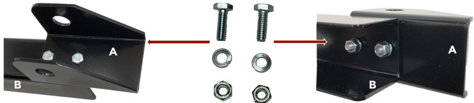
TOP VIEW: Use the 2) 1/4" x 3/4" bolts and insert them thru both holes with the receiver mount base
