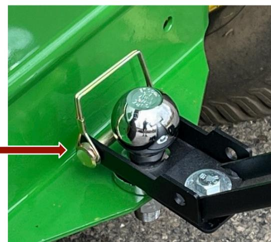
**Step 2- Mount the 2) mountain hooks and 2) retainer bracket to the support arm**
