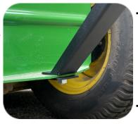
Bolt the support arm (B) using the  $7/16" \times 1"$  bolt (H) Bolt on to the flange of your tow vehicle, using the under side support washer (F) on the bottom of the vehicles flange. This will help stiffen the mounting flange
